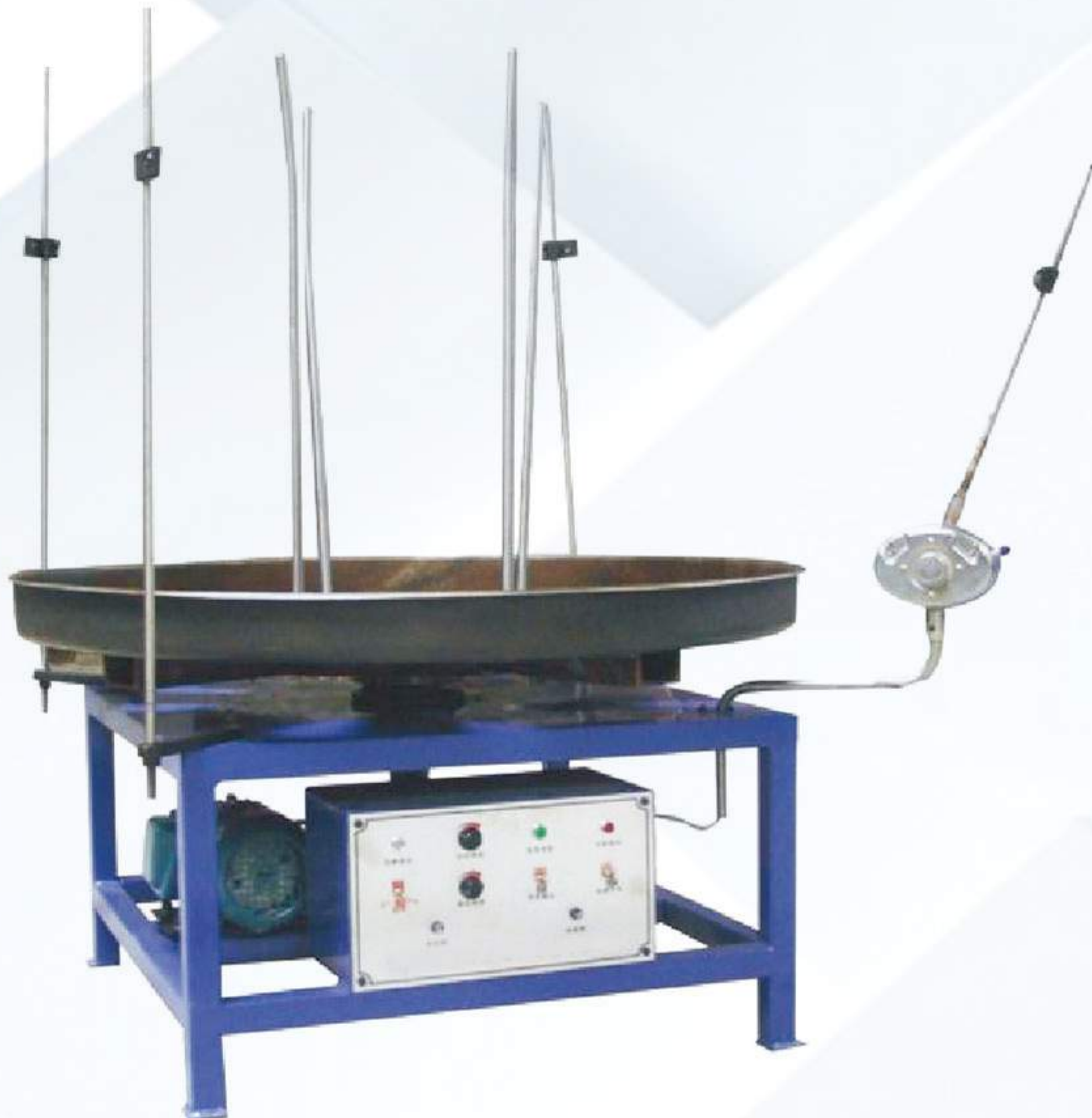
Automatic material feed frame
